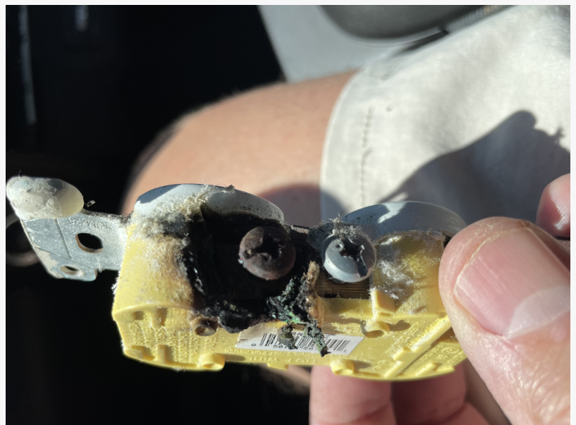
Loose Wiring Is A Fire Hazard!
