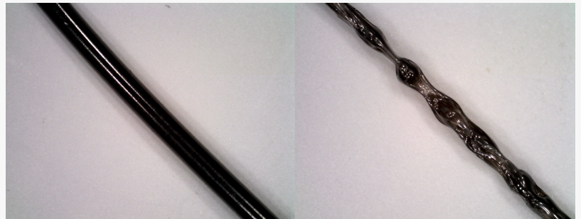
A micrograph of a laminar ABS extrudate is compared to a bead that was printed too fast and too hot, resulting in melt fracture.
