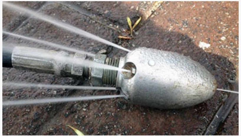
high pressure hydro jetting by the Los Angeles Grease Co.
