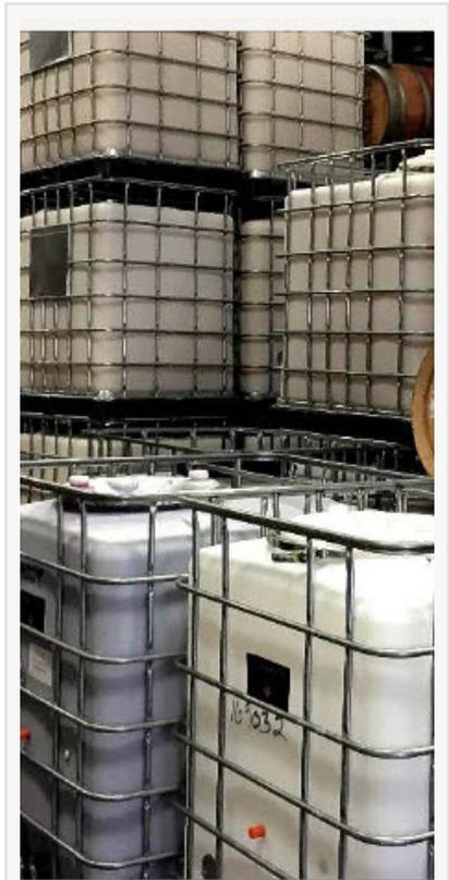
Flextanks help wineries increase capacity, and reduce costs. Flextanks deliver controllable, stackable, sustainable production via adjustable oxygen-permeable surface area-to-volume ratio and related wall thickness and configuration.
