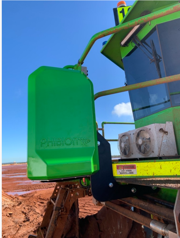
Real time density sensor attached to the MudMaster in Western Australia
