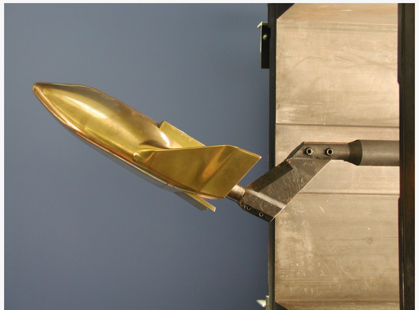
This model of the X-38 spacecraft was examined in the RWG system on behalf of ESA and NASA. Source: DLR.
