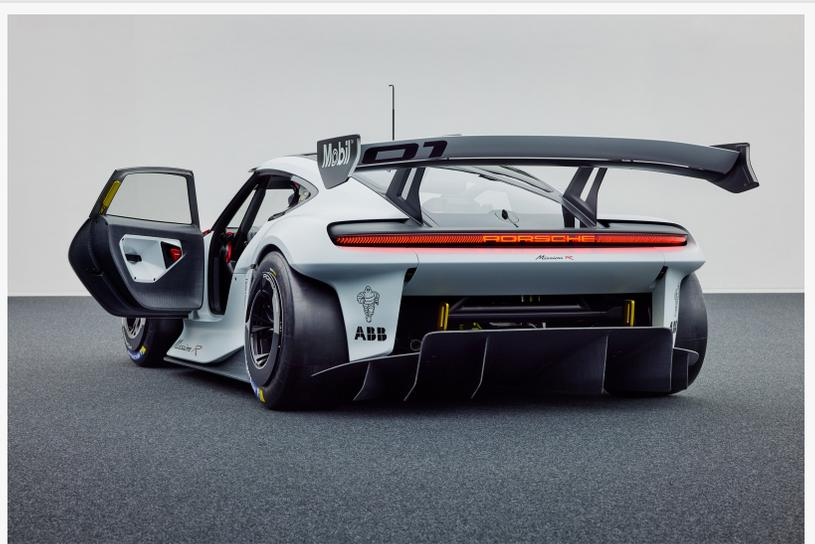
Many of the add-on parts on Porsche's visionary fully electric Mission R concept car are made using Bcomp's natural fibre reinforced plastic, including front splitter, the doors, the side skirts and diffuser.
