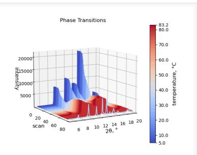
X-ray diffraction patterns of theophylline monohydrate (Theo-FM) held at 5% rH collected between 5 °C and 83 °C. Conversion from the monohydrate to a metastable form occurs (Theo-Meta). At 55 °C the Theo-FM disappears. Theophylline Form II (Theo-F2) appears at 40 °C.
