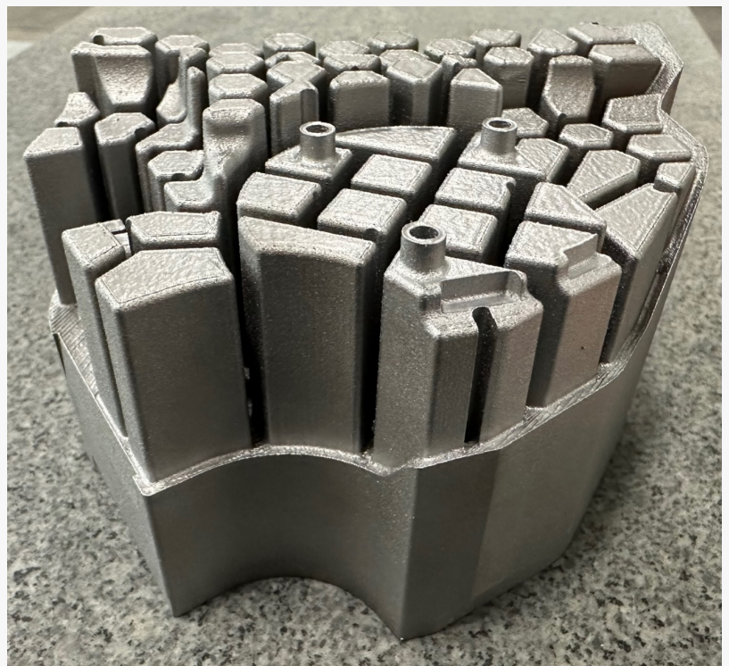
HTC-45 Core Insert With Conformal Cooling
