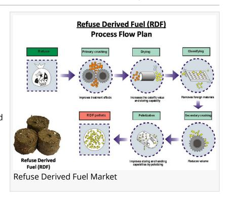
Refuse-derived fuel (RDF) is extracted from municipal solid wastes, and commercial wastes or industrial wastes. The production of RDF can minimize the potential of methane emissions in atmosphere and to minimize the pressure on landfills.
