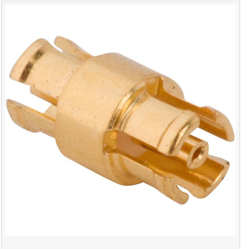
[SMPM bullet adapters](#) are machined from beryllium copper with gold plating for high-frequency electrical performance. When used in conjunction with SMPM PCB connectors, this three-piece design is well-suited for blindmate situations. This series is available in straight and right-angle configurations with cable solutions optimized to meet the frequency limits of high-frequency cables, and PCB options with surface mount, through-hole leg or edge mount terminations.
