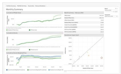
REview helps customers understand settlement impacts potentially caused by a project's operations by comparing modeled settlement to actual settlement.
