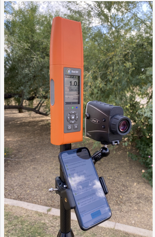
Bad Elf Flex with LTI Rangefinder and Esri ArcGIS Field Maps
