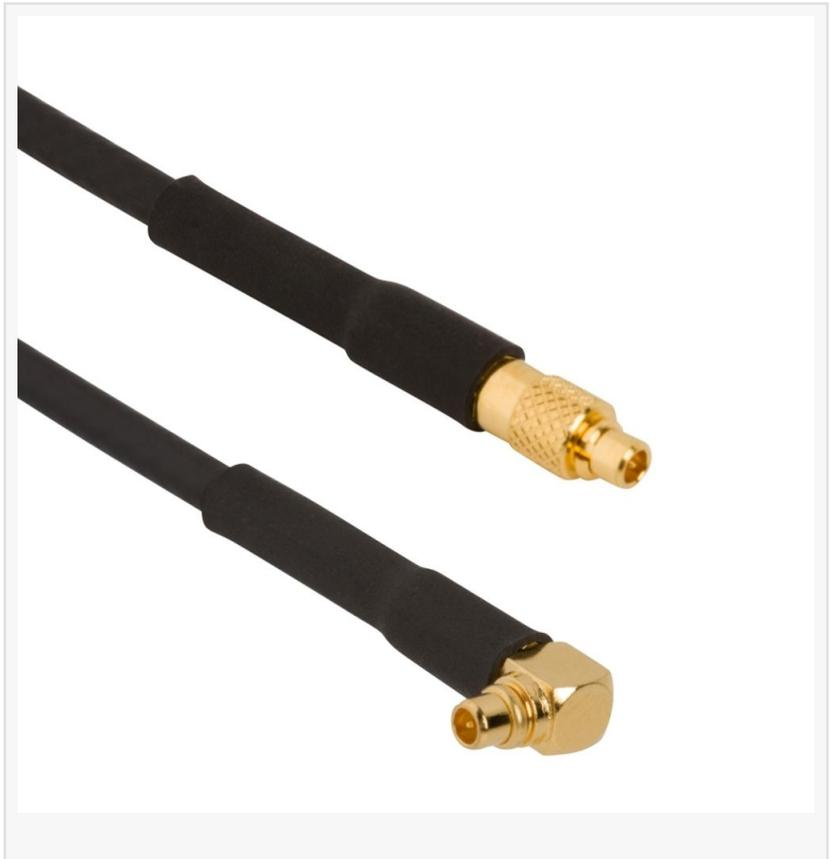
The MMCX connector series is a robust micro-miniature interface with broadband capabilities up to 6 GHz. They feature the reliable snap-on/snap-off coupling mechanism for quick and easy mating. These connectors are manufactured from brass with gold plating and offer reliable electrical performance up to the limits of the cable type. Their small size paired with the flexible cable types make them an ideal choice for compact applications.
