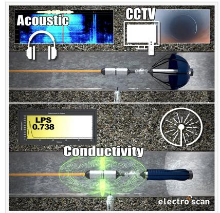
Multi-sensor probe combines Acoustic (legacy listening), CCTV (visual navigation), and Conductivity (pinpoint leak location), in a single in-pipe tethered platform.
