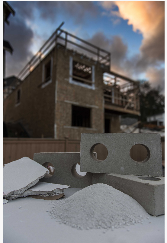
Drywall Waste Blocks are shown alongside scrap drywall and the gypsum powder made from processing the scraps
