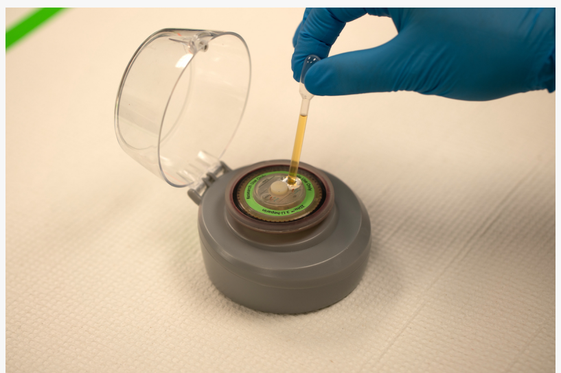
Sandstone's Torq Zero Delay Centrifuge System enabling decentralized blood sample collection and sample preparation
