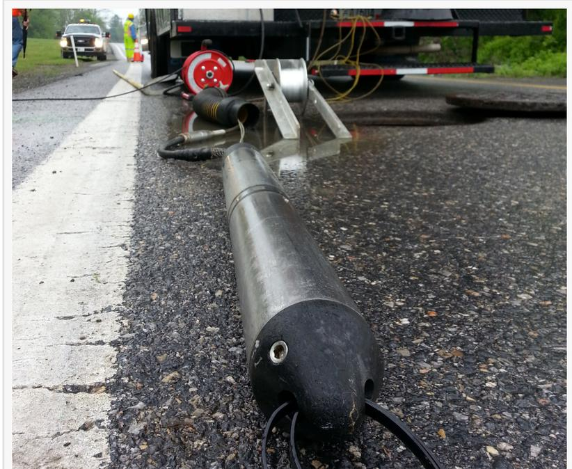
Electro Scan ruggedized machine-intelligent pipeline assessment probe.
