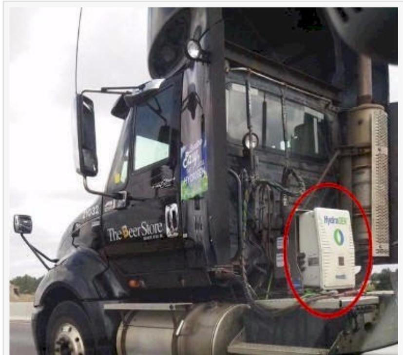
dynaCERT HG unit installed on diesel Truck
