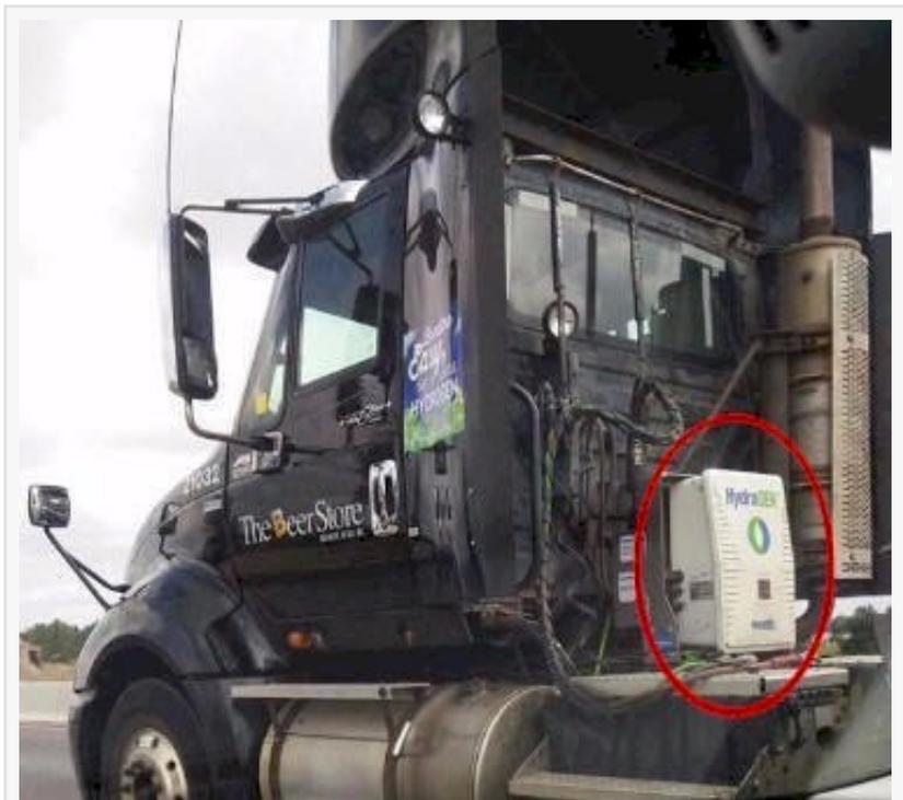
dynaCERT HG unit installed on diesel Truck
