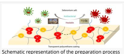
Schematic representation of the preparation process of PUa-C7 Seb+ materials.
