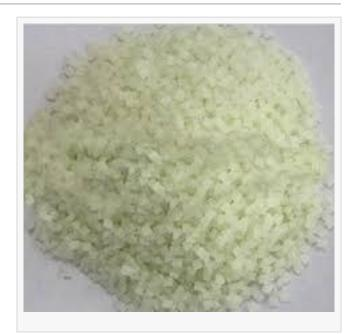
advantages of High performance polyamide includes high melting point, reduced absorption of moisture, and better retention of mechanical properties at high temperature. The fibers of such polyamides are manufactured in various forms like textile filament, or as industrial filament.
