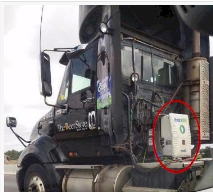
dynaCERT HG unit installed on diesel Truck
