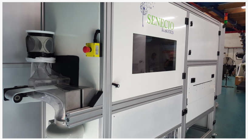
Loading station loading measured number of mosquitoes per each release box mounted at the loading position
